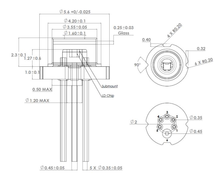
Note : Tolerance is  $\pm 0.05$ mm for items without tolerance marking
